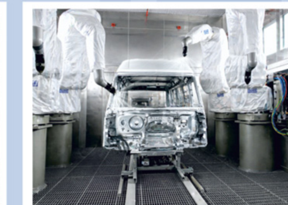
Robotic painting for car-like gloss and even paint finish
