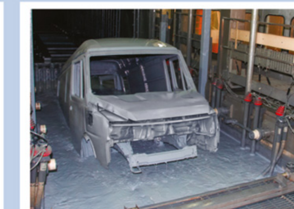
7th Generation CED painting for unmatched corrosion resistance
