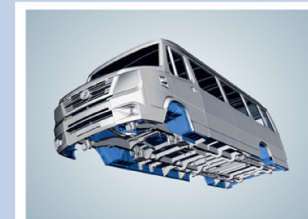
Monocoque design for outstanding structural strength
