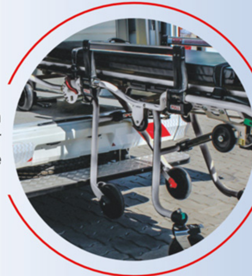
Mounting provision on floor to secure stretcher in moving vehicle
