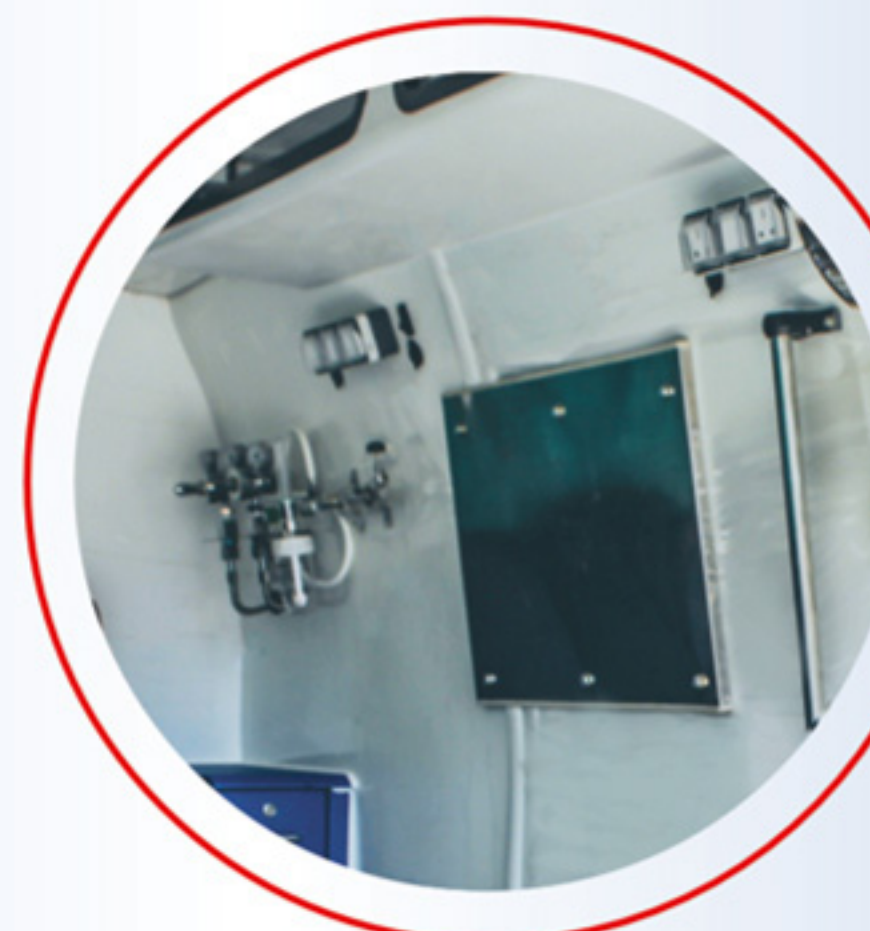
Oxygen delivery system and stainless steel plate to mount defibrillator, ventilator, suction pump, etc.
